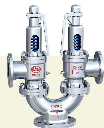
HFA38系列双联弹簧式安全阀 HFA38 Series duplex spring safety valve 使用介质: 蒸汽 Medium: Steam Std.:GB/T 12243 Sizes: DN50~150 Press.: PN16 ~ 40 Temp.: -29°C ~ 350°C
