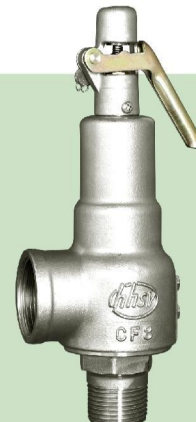
HFA28系列弹簧式安全阀 HFA28 Series spring safety valve 使用介质: 气体、蒸汽 Medium: Gas, steam Sizes: 1/2"-2" Press.: Class 150Lb ~ 300Lb Temp.: -196°C ~ 300°C
