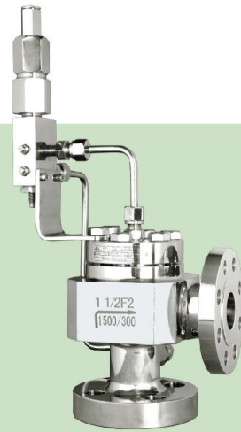
HFXD系列先导式安全泄压阀 HFXD Series pilot operated safety relief valve 使用介质: 气体、液体 Medium: Gas, liquid Std.:ASME VIII-API 526 Sizes: 1"-10" Press.: Class 150Lb ~ 2500Lb Temp.: -196°C ~ 200°C
