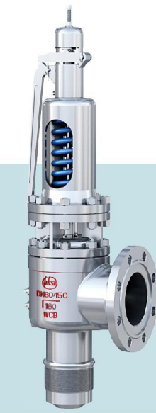
HFGS系列焊接型弹簧式安全阀 HFGS Series welded type spring loading safety valve 使用介质: 蒸汽 Medium: steam Std.:ASME I Sizes: 2"-10" Press.: Class 600Lb ~ 2500Lb Temp.: 300°C ~ 540°C
