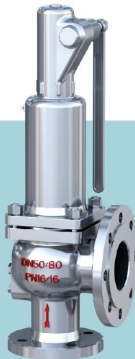
HFA900系列弹簧式安全阀 HFA900 Series spring safety valve 使用介质: 气体、液体、蒸汽 Medium: Gas, liquid, steam Sizes: 3/4"-8" Press.: Class 150Lb ~ 300Lb Temp.: -196°C ~ 300°C
