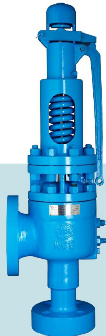
HFGS系列弹簧式高温蒸汽安全阀 HFGS Series high temperature spring safety valve 使用介质: 蒸汽 Medium: steam Std.:ASME I Sizes: 1 1/2"-8" Press.: Class 150Lb ~ 2500Lb Temp.: -29°C ~ 565°C
