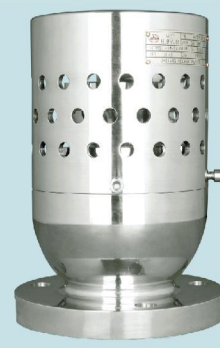
HFA72W系列真空负压安全阀 HFA72W Series vacuum negative pressure safety valve 使用介质: 气体 Medium: Gas Sizes: 1/2"-10" Press.: Class 150Lb Temp.: ≤200°C
